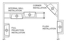
Figure 1 - Possible Locations for Installing Appliance
